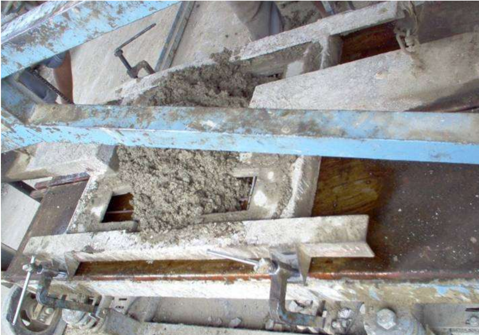
Pouring in concrete over the mould.
