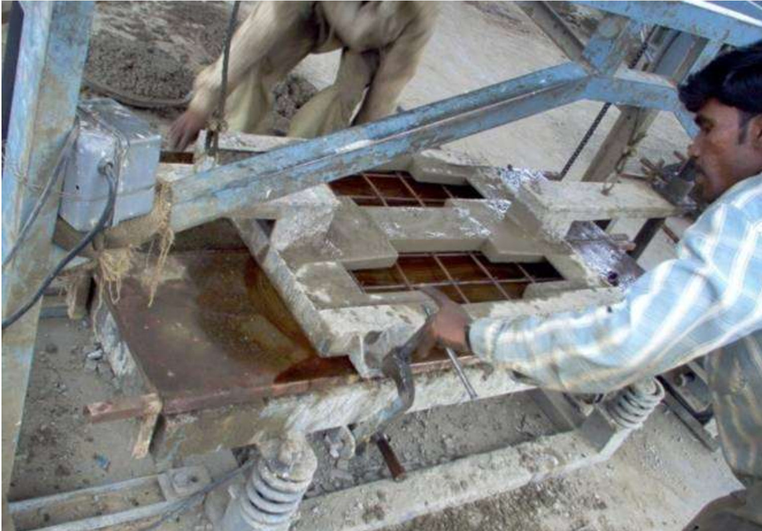
Locking the mould in position over the trays.
