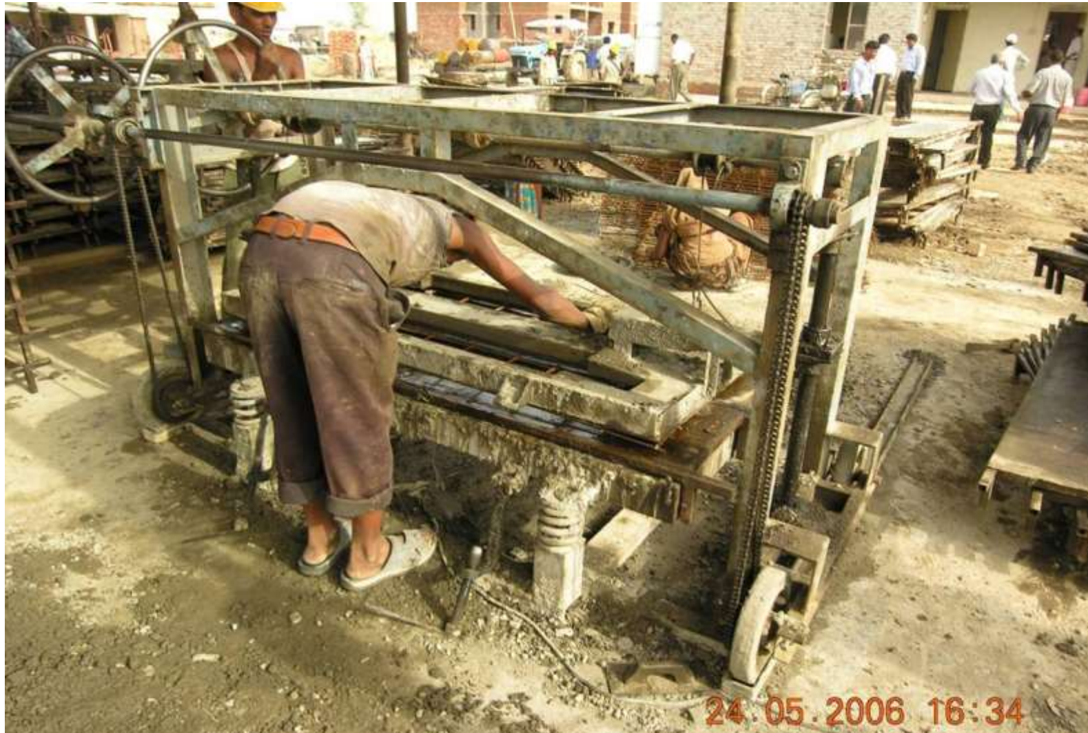
Locking the mould in position over the trays.
